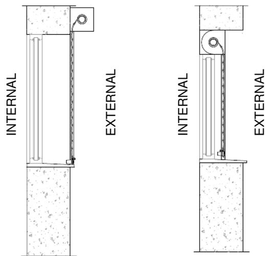
**Figure 2. Section through external blind installation: retrofit (left), compact (right)**
