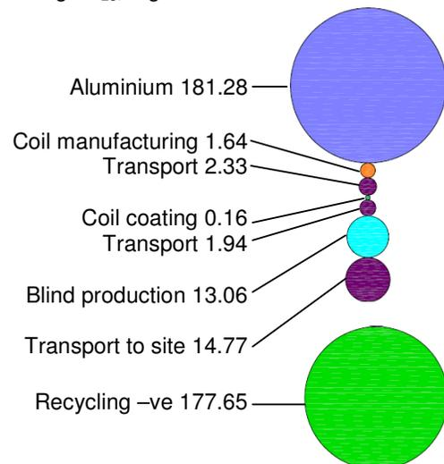
Figure 7. LCA processes and emissions quantities (kgCO<sub>2e</sub>)
