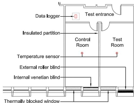
**Figure 4. Floor plan of concept study**
